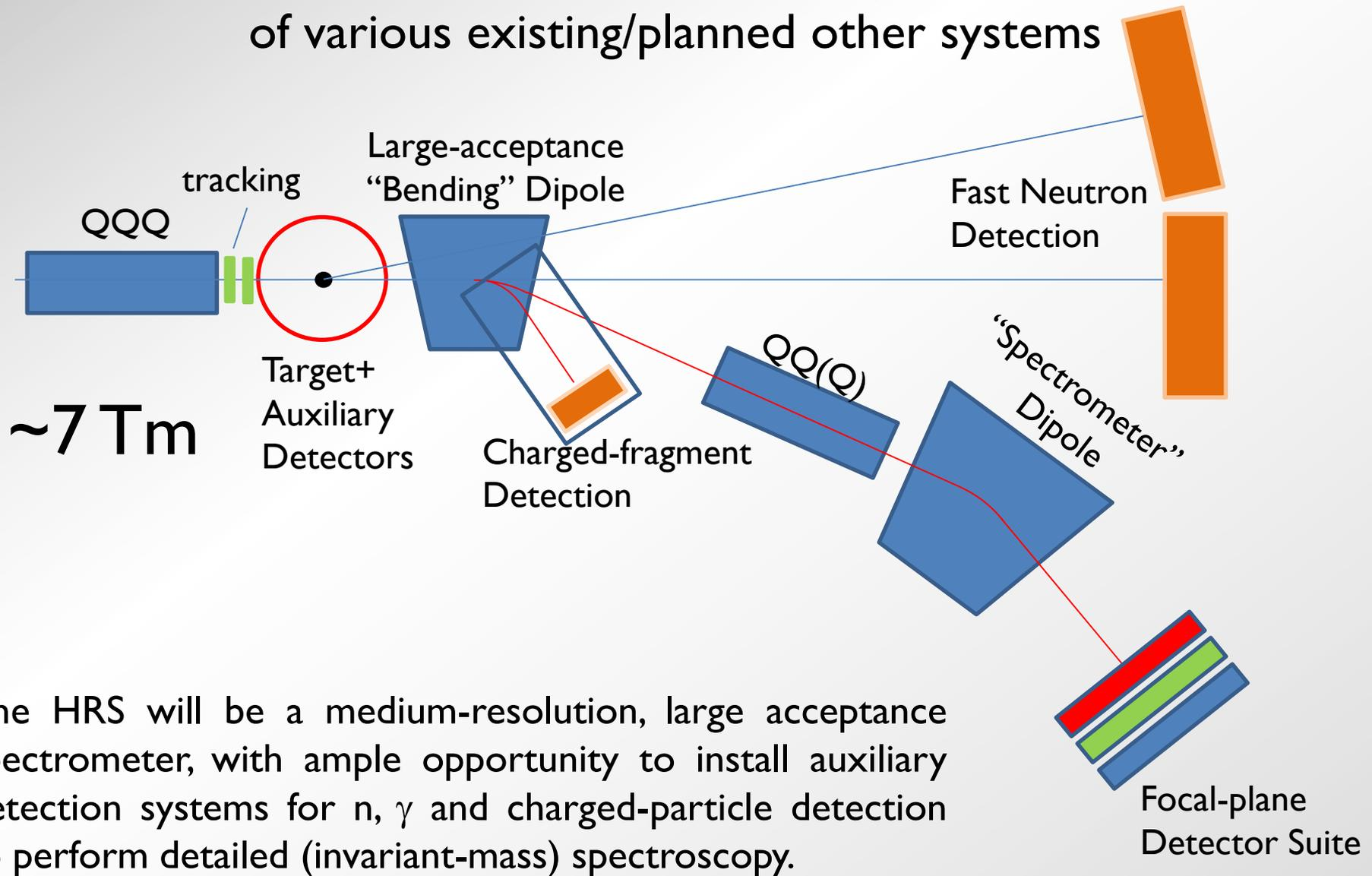
The HRS will be a medium-resolution, large acceptance spectrometer, with ample opportunity to install auxiliary detection systems for  $n$ ,  $\gamma$  and charged-particle detection to perform detailed (invariant-mass) spectroscopy.
