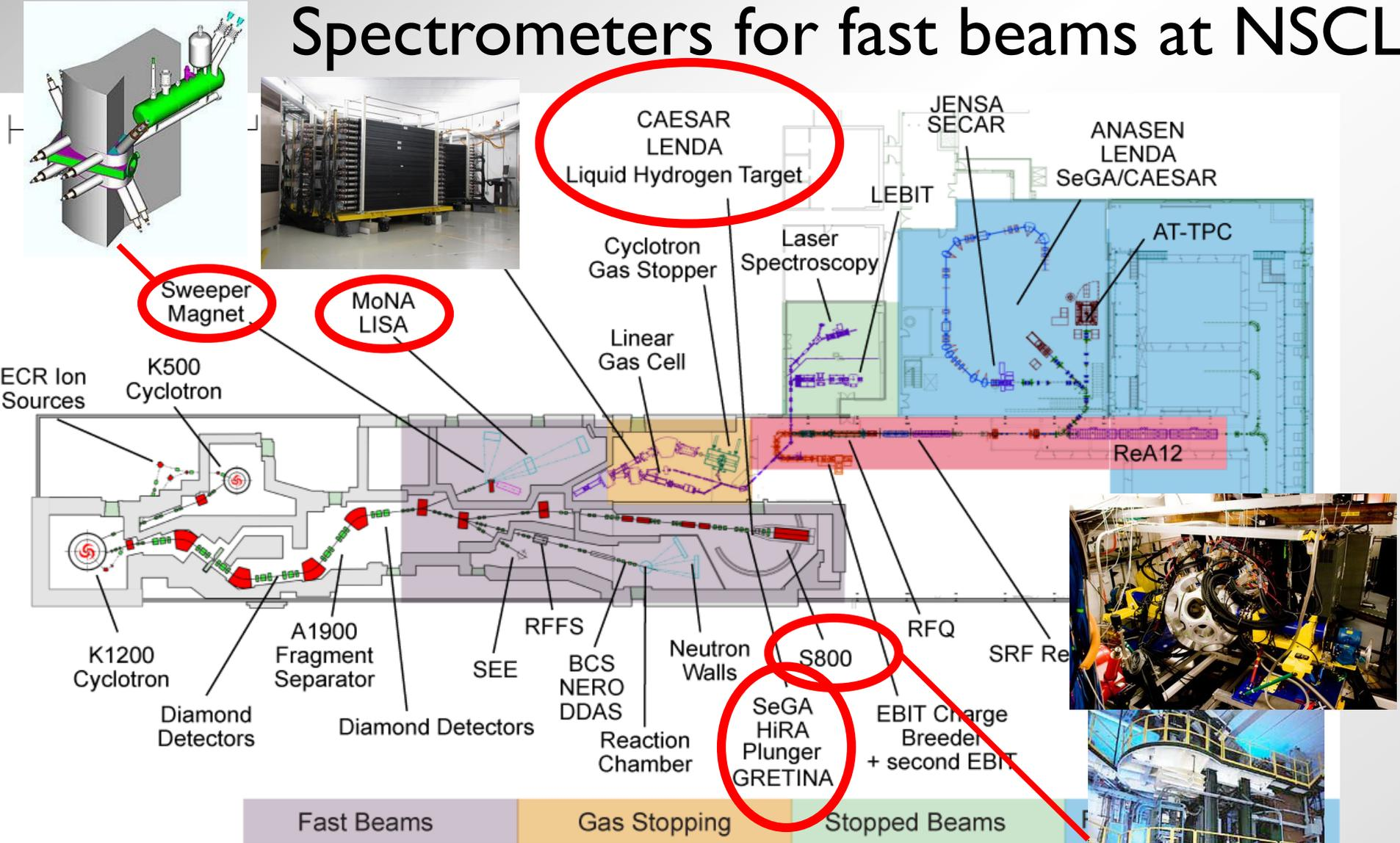
The magnetic rigidity of the S800 and Sweeper are limited to  $\sim 4 \text{ Tm}$ .
