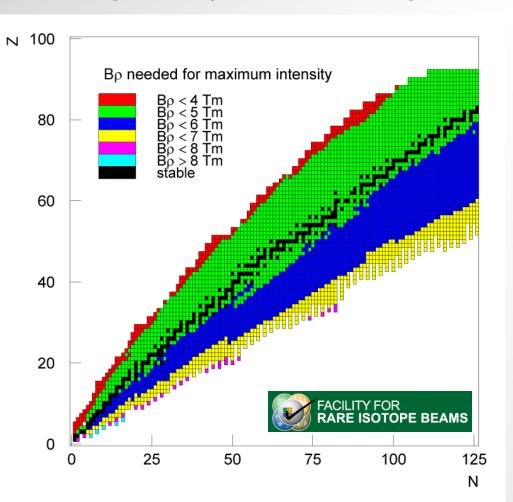
Optimum rigidities for performing experiments with neutron-rich rare isotopes are beyond the capabilities of the S800 and Sweeper magnets.
