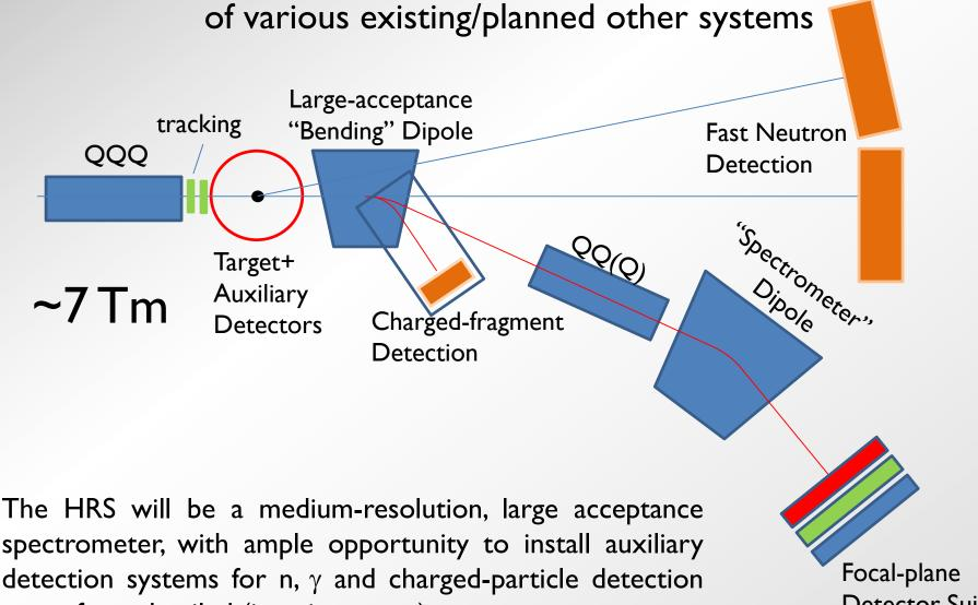
spectrometer, with ample opportunity to install auxiliary detection systems for n,  $\gamma$  and charged-particle detection to perform detailed (invariant-mass) spectroscopy.
