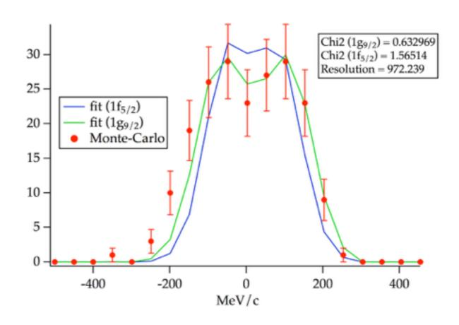
Simulation of the longitudinal momentum distribution of <sup>89</sup>Zr from the neutron knockout of <sup>90</sup>Zr, assuming the valence neutron is either in the If<sub>5/2</sub> or Ig<sub>9/2</sub> orbital. A resolution of I/1000 in momentum is needed to identify the angular momentum from the shape of the simulated Ig<sub>9/2</sub> momentum distribution.
