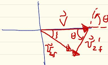
$$\begin{aligned} Y: \quad V_4 \sin \xi &= V_{2f}' \sin \theta \\ X: \quad V_{2f} \cos \xi &= V - V_{2f}' \cos \theta \end{aligned} \quad \Rightarrow \quad \tan \xi = \frac{\sin \theta}{\left( \frac{V}{V_{2f}'} \right) - \cos \theta}$$
