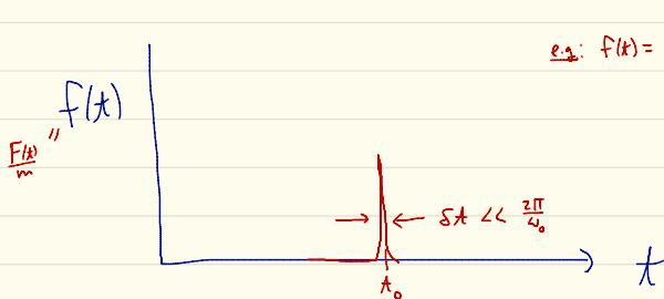
$$\text{e.g.: } f(t) = \begin{cases} 0 & t < t_0 \\ \frac{V_0}{\Delta t} & \text{if } t_0 \leq t \leq t_0 + \Delta t \\ 0 & \text{if } t > t_0 + \Delta t \end{cases}$$
