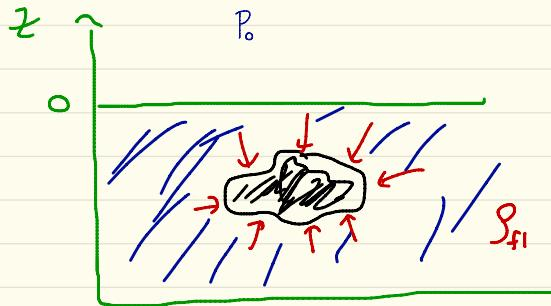
Archimedes Principle: Buoyant force = weight of displaced fluid applied @ CM of displaced fluid
