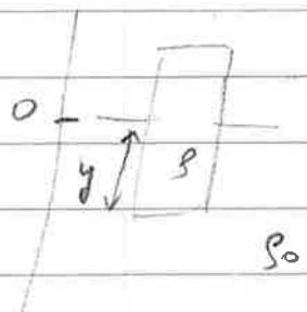
$$(b) \quad v_o = \frac{1}{2\pi} \sqrt{\frac{9.81 \frac{m}{s^2} \times 1}{0.03m \times 0.8}} = 3.2 \text{ Hz}$$
