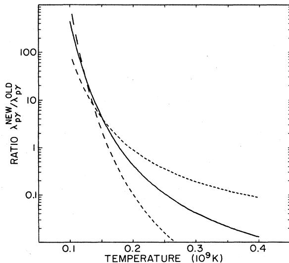
FIG. 5. The ratio of the recalculated  $^{56}\text{Ni}(\text{p},\gamma)^{57}\text{Cu}$  rate in units of  $\text{cm}^3/\text{mole sec}$  to the previously calculated rate versus temperature. The dashed lines were calculated by varying the resonance energy by the uncertainty in the measurement,  $\pm 40$  keV.
