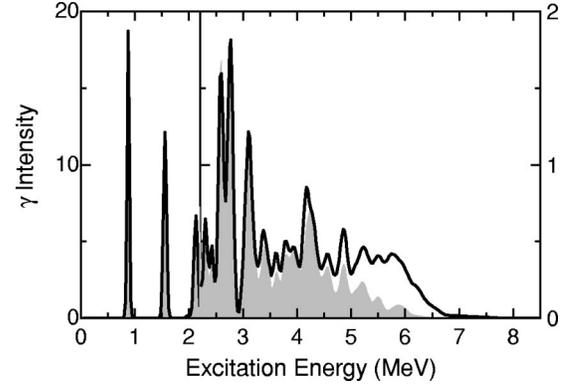
FIG. 5. Gamma intensity for the  $\beta$  decay of  $^{98}\text{Ag}$  as a function of  $^{98}\text{Pd}$  excitation energy, derived from TAS data (solid line) and from the Cluster Cube measurement (shaded area). The  $\gamma$  intensity is defined as the number of quanta emitted per  $\beta$  decay, integrated over an excitation-energy interval of 1 MeV. The ordinate scale is reduced by a factor of 10 for excitation energies above 2.2 MeV.
