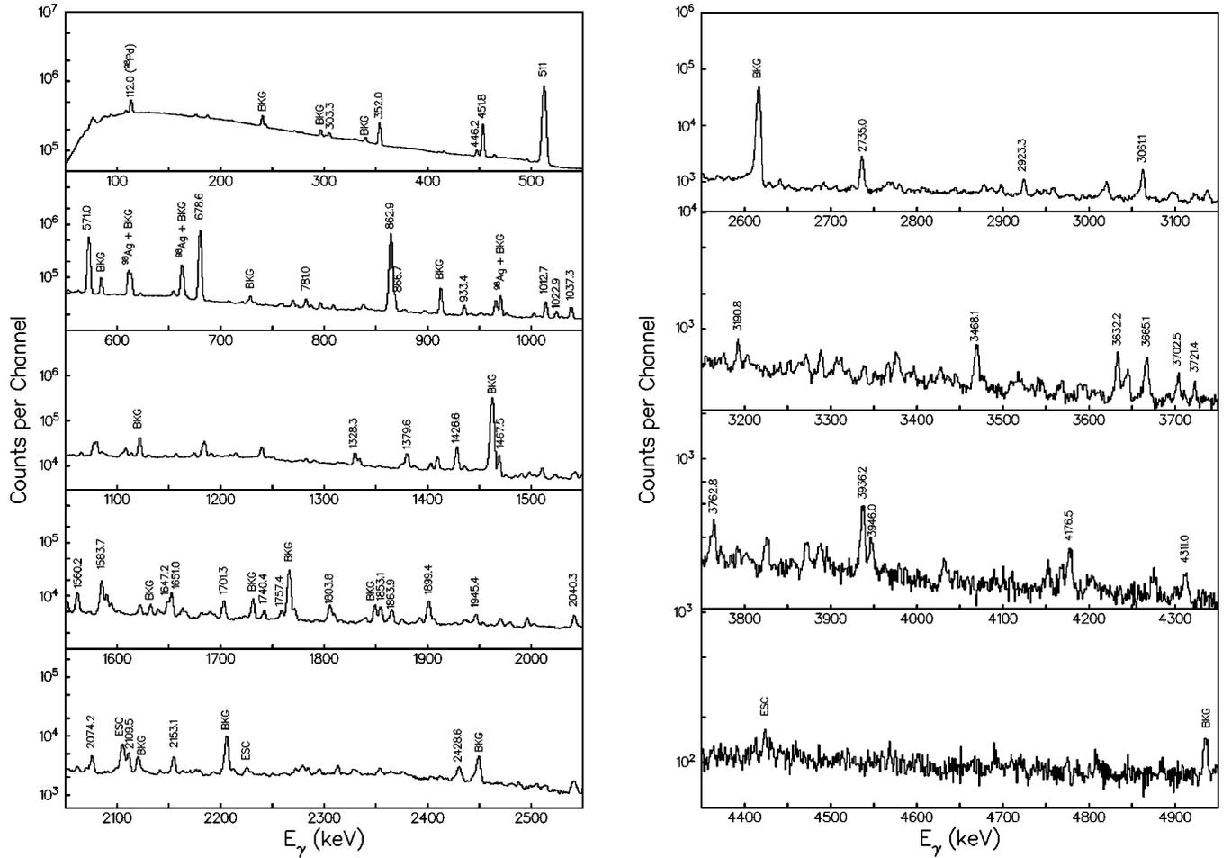
FIG. 1. Gamma-ray singles spectrum obtained by using the 42 capsules of the Cluster Cube for the measurement of mass-98 samples. See text for details.
