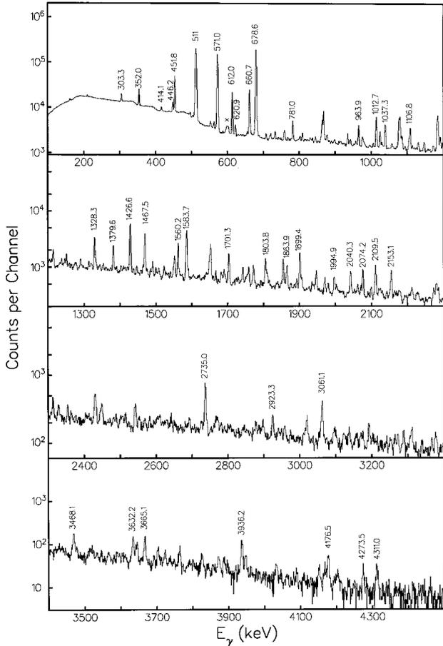
FIG. 2. Background-subtracted coincidence spectrum from the Cluster Cube data, gated on the 862.8 keV  $\gamma$ -ray transition. See text for details.
