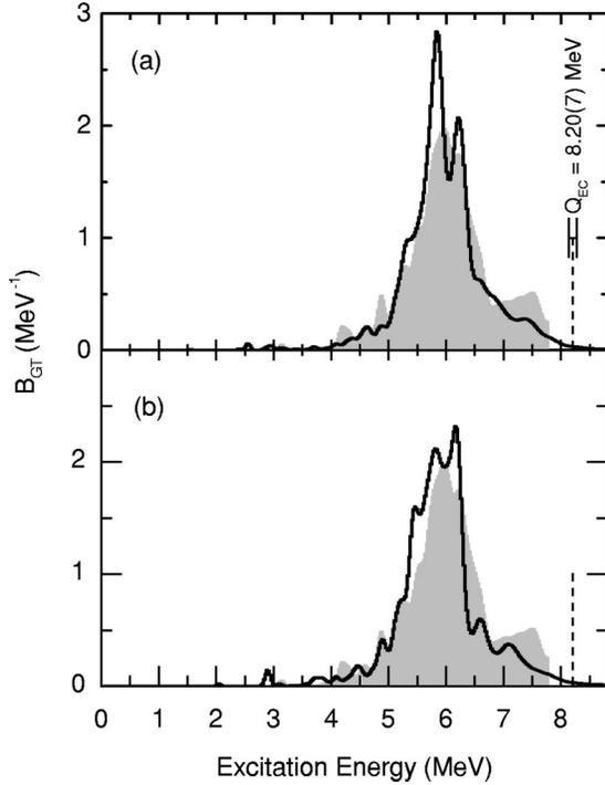
FIG. 7. GT-strength distributions for the decay of  $^{98}\text{Ag}$  obtained from the TAS measurement (shaded area) and from the SNC shell-model calculation (solid line) assuming the  $^{98}\text{Ag}$  ground-state spin of  $5^+$  (a) and  $6^+$  (b). The theoretical GT strength has been reduced by a hindrance factor of 4.6.
