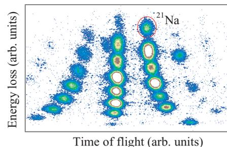
FIG. 1. (Color online) Identification of the  ${}^{20}\text{Ne} + {}^9\text{Be}$  projectile-like reaction residues in the S800 focal plane, shown as the energy loss measured in the ionization chamber versus the ion's time of flight. The  ${}^{21}\text{Na}$  one-proton pickup residues are clearly separated from the other reaction residues.
