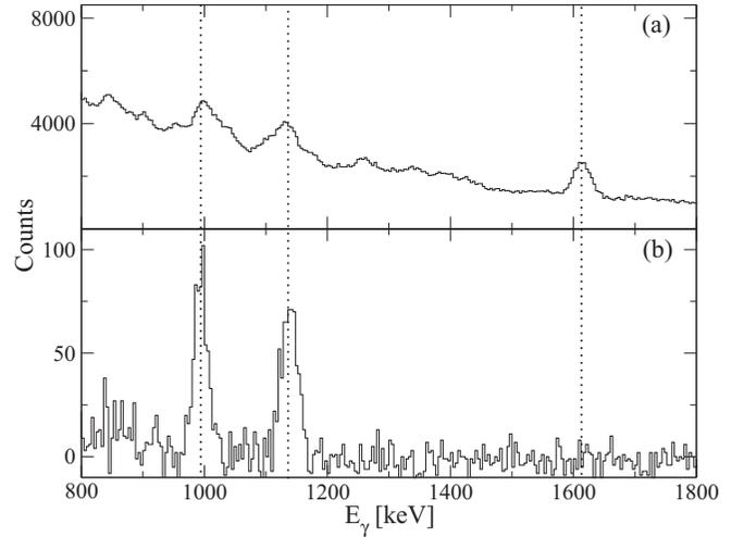
FIG. 3. The  $\gamma$ -ray energy spectra measured in the  $\text{LaBr}_3(\text{Ce})$  detectors: (a) The total projection of the  $E_\gamma$ - $E_\gamma$  matrix with gates in the HPGe detectors on the 140-, 225-, 246-, and 413-keV transitions, and (b) with the addition of a gate on the 1609-keV transition in a  $\text{LaBr}_3(\text{Ce})$  detector. The dashed lines indicate the positions of the feeding (992- and 1132-keV) and deexciting (1609-keV) transitions for the  $\frac{13}{2}^+$  state.
