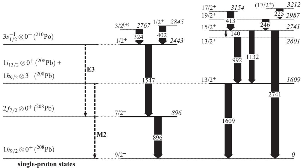
FIG. 1. The partial level scheme of the low-lying states in  $^{209}\text{Bi}$ . The dashed lines represent the pure multipole transitions, for which strengths are extracted in this work. The transition energies are given in keV and the width of the arrows represents the intensity of the transitions normalized to 100% for the strongest transition from each level [21]. The thicker lines denote the levels for which decay spectra were analyzed in this work.
