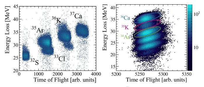
FIG. 2. Left: Energy loss vs TOF identification of the nuclei produced along with <sup>37</sup>Ca. Right: Identification of heavy transfer residues from their energy loss, measured in the ZDD ionization chamber, and their time of flight measured between the first CATS detector and the plastic scintillator located at the end of the ZDD (see text for details). The blue, purple and green contours show the regions corresponding to outgoing Ca, K, and Ar nuclei, respectively.
