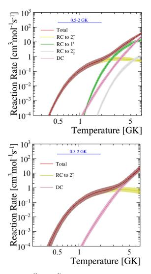
FIG. 6. The  ${}^{35}$ K( $p, \gamma$ )  ${}^{36}$ Ca reaction rate calculated (in units of cm<sup>3</sup> mol<sup>-1</sup> s<sup>-1</sup>) in this work (top) and in Ref. [16] (bottom). The red curve represent the total reaction rate, which includes the contributions of resonant (RC) and direct (DC) captures. The thickness of the curves represents a coverage probability of 68%. The indicated range of 0.5–2 GK is typical of x-ray burst temperatures.
