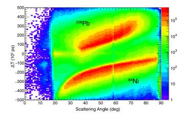
FIG. 1. Time-of-flight difference between the projectile and target recoils as a function of scattering angle measured with the CHICO2 detector. A clear separation between the <sup>64</sup>Ni (bottom) and <sup>208</sup>Pb (top) ions is observed.
