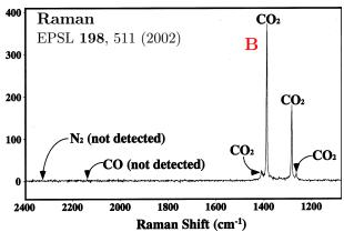
2. Let us now consider  $CO_2$  as a classical tri-atomic molecule. To perform molecular spectroscopy, samples are exposed to (nearly) monochromatic radiation to excite their molecular normal modes. The changing fields of the electromagnetic waves can be viewed as a periodic driving force with a (nearly) unique external frequency  $\omega_{\text{ext}}$ .
