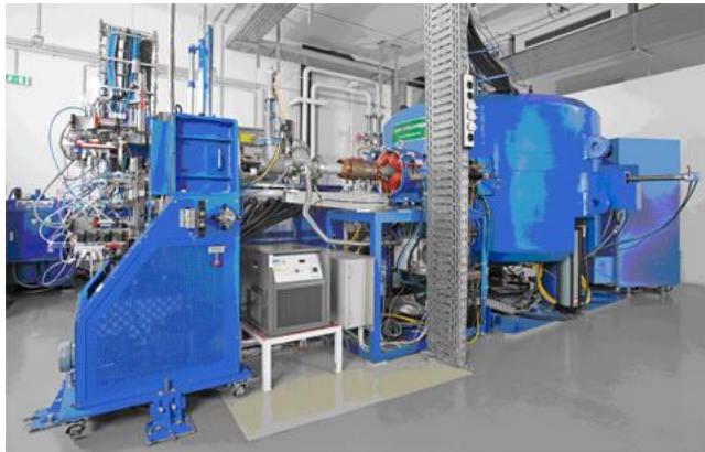
Left: 17 MeV GE PETtrace cyclotron
