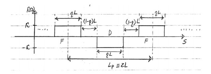
$$\begin{split} L_p &= 2L = \text{Lattice period} \\ \eta L &= \text{Quadrupole length} \\ (1 - \eta)L &= \text{Drift length} \\ \eta &= \text{Quadrupole occupancy} \ , 0 < \eta \leq 1 \\ \kappa &= \text{Quadrupole strength} \end{split}$$
