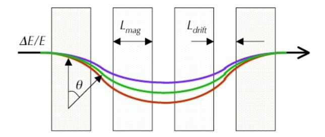
A "chicane" consists of four identical sector dipoles as shown above. Each dipole has axial length  $L_{\text{mag}}$  and bends the beam by angle  $\theta_B$ . The drift space between two adjacent dipoles is  $L_{\text{drift}}$ . Show for the chicane lattice that:
