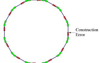
If the particle is oscillating with integer tune, then the particle experiences the dipole error on each lap in the same oscillation phase and the trajectory will "walk-off" on a lap-to-lap basis in phase-space:
