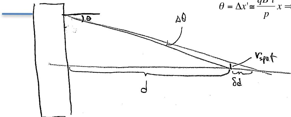
$$\begin{aligned} r_{\text{spot}} &= \theta \delta d \\ &= \theta \frac{\delta d}{\Delta \theta} \frac{\Delta \theta}{\Delta p} \delta p \\ &= \alpha \theta d \left( \frac{\delta p}{p} \right) \end{aligned}$$
