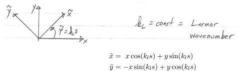
Find an expression for  $k_l$  to reduce the equations of motion to the decoupled form:
