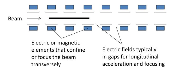
This array or "lattice" of focusing elements may be arranged in a linac or circular accelerator
