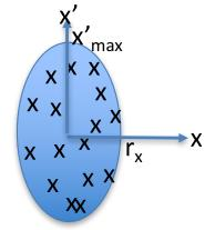
For non-accelerating paraxial beam x' proportional to  $p_x$ , etc.
