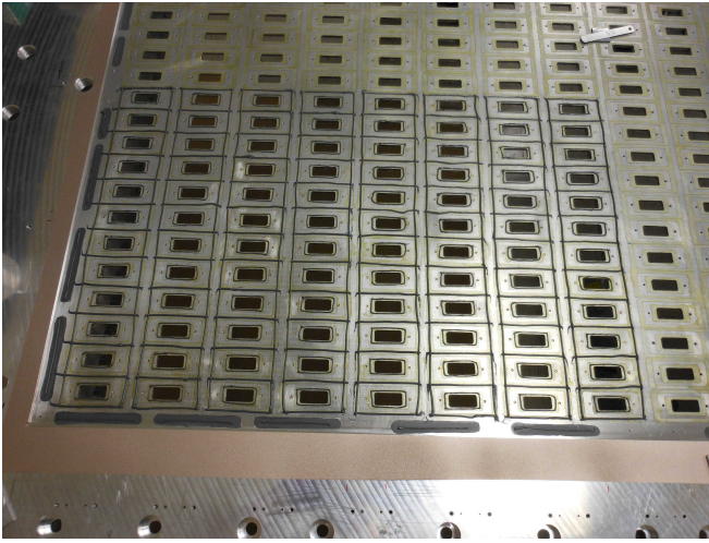
FIG. 8: Photograph of the top plate and glue pattern prior to gluing the pad plane to the top plate. The dark rectangular lines are the Araldite 2013 glue beads.
