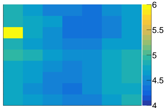
FIG. 18: Typical noise level of pads within the unit cell, with noise level in ADC channels. The orientation of the pads matches that of Fig. 7.
