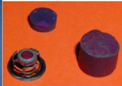
cathodes damaged by sputtering (see later)
