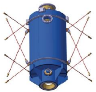
Figure 4.120: Helium vessel with hanging rod
