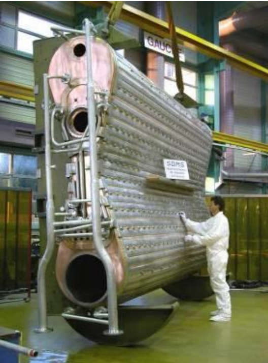
CW 50.6 MHz cavity of PSI cyclotron. V = 1.2 MV
