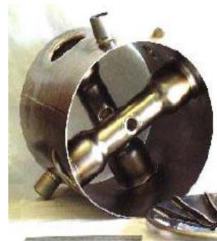
345 MHz, \beta=0.4 , 3-gap spoke cavity for ion beam acceleration ANL
