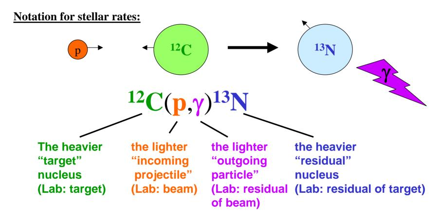
(adapted from traditional laboratory experiments with a target and a beam)
