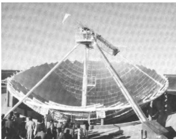
Figure 3-8. Analog Design Verification System 20-m Bowl Collector
