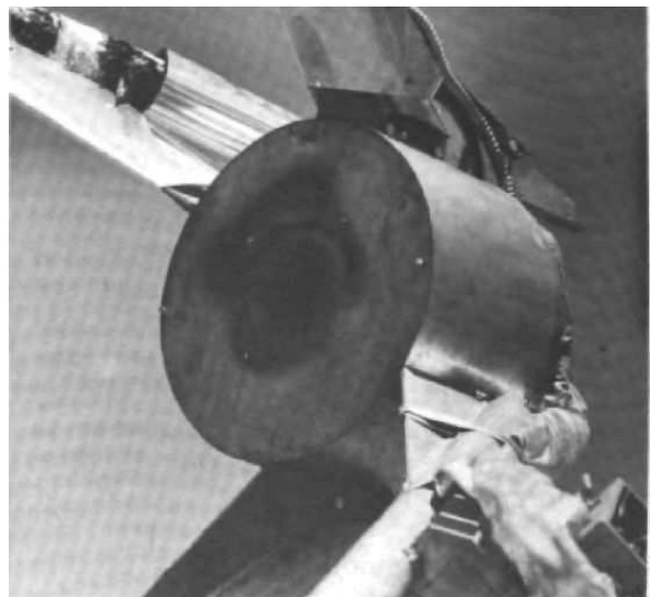
Figure 4-4- Advanced Thermal Receiver Under Test at SERI
