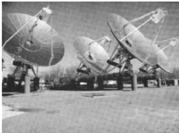
Figure 1-25. Shenandoah Collector Prototypes at the Midtemperature Solar Systems Test Facility
