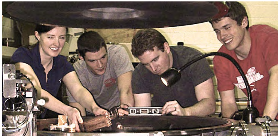
Figure 4. Post doctoral associate Kate Blesener, undergraduate student Elliot Rosenberg, and graduate students Cad Hoyt and Peter Schrafel insert and level an x-ray spectrometer in the COBRA vacuum chamber for high energy density z-pinch experiments.
