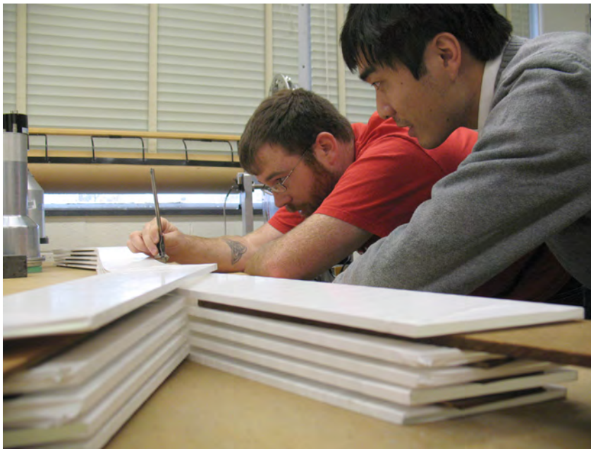
Figure Caption 1. The individually wrapped scintillator layers, and their Y-shaped light guides.
