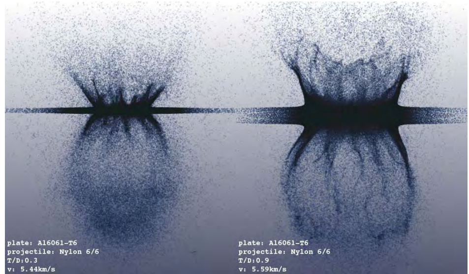
Figure 1. Example of simulation of two hypervelocity-impact experiments performed under the auspices of Caltech's PSAAP Center. A nylon 6/6, 1.67 mm diameter and length, cylindrical projectile strikes Al6061-T6 aluminum plates of two different thicknesses, 0.5 mm (left) and 1.5 mm (right), at 5.44 km/s (left) and 5.59 km/s (right), thereby setting in motion complex physics ranging from an initial impact plasma to fragmentation and debris-cloud formation. The complexity of the material behavior and attendant deformation process render this type of simulation a predictive challenge, and tests the limits of our ability to predict material behavior under extreme conditions. The figures show predicted shadowgraphs showing the structure of the debris cloud in a manner that lends itself to direct full-field, 3D comparisons with experimental data.
