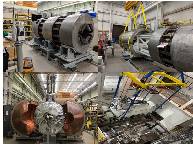
Cold Iron Quad Triplet for FRIB Fragment Separator, FRIB, MSU
