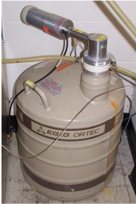
Standard Ge detector available for this class. Value: several $10,000
